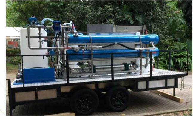
Skidframe RO unit 275m 3 /d, permeat staged
